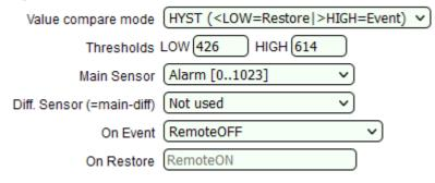
The idea of this setting is that when the value of the alarm input (in practice it is an analog input with a value from 0 to 1023) exceeds 614 (this is equivalent to an **open** contact) the macro "Remote OFF" will be launched once. The relay of device "B" will switch off and its normally open contact on Line 1 will be **open**.
