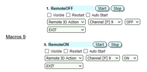
At this stage you can perform a manual test with the Start buttons for both macros: you must register the change in the state of the relay of Line 1 on device "B". If this does not happen - there is a problem in the network and / or SNMP settings.
